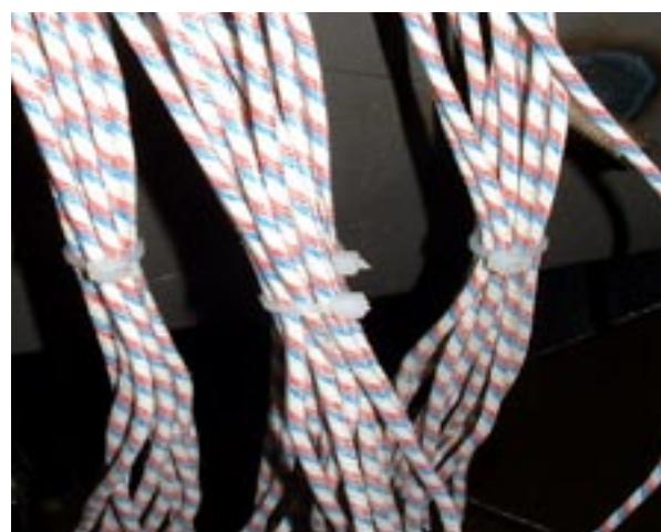
In order to make easier the connection, mark and attach the wires of resistances by group
