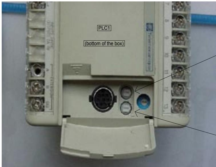
Potentiometer to adjust the first fold (normal folding)
